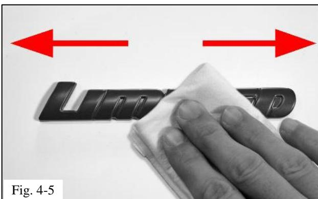
(e) Using a lint-free scratch resistant cloth, press firmly on the emblem cap from the center working outwards to the edges of the emblem cap, to ensure maximum adhesion contact (Fig. 4-5).
