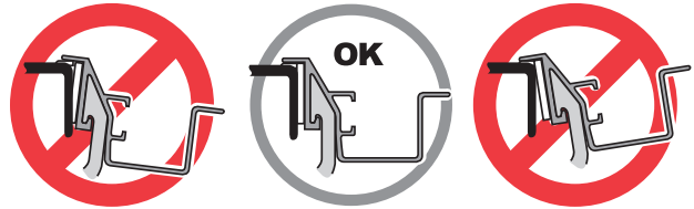
Clamp too low pulling side rail down
